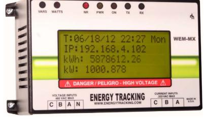
This version of the WEM-MX uses 333 millivolt "safe" current transformers—reducing cost, improving installation flexibility, and significantly reducing risk of shock to installation or service personnel.
