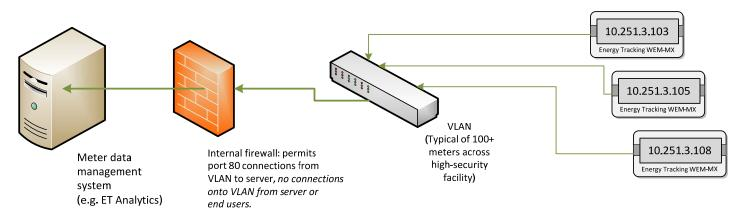
A typical network installation: the internal building firewall blocks all inbound access; meters are isolated on a standard virtual local-area network (VLAN). This is a typical default firewall configuration—and does not present the network security issues, and ongoing firewall maintenance, that legacy polling protocols (e.g. Modbus, BACNet) require.
